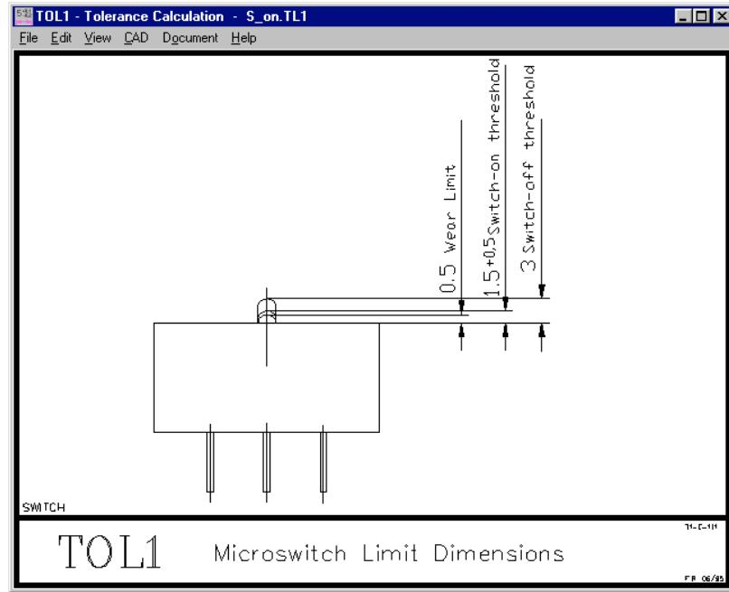
For safe use the switching zone for the actuator is as follows:
