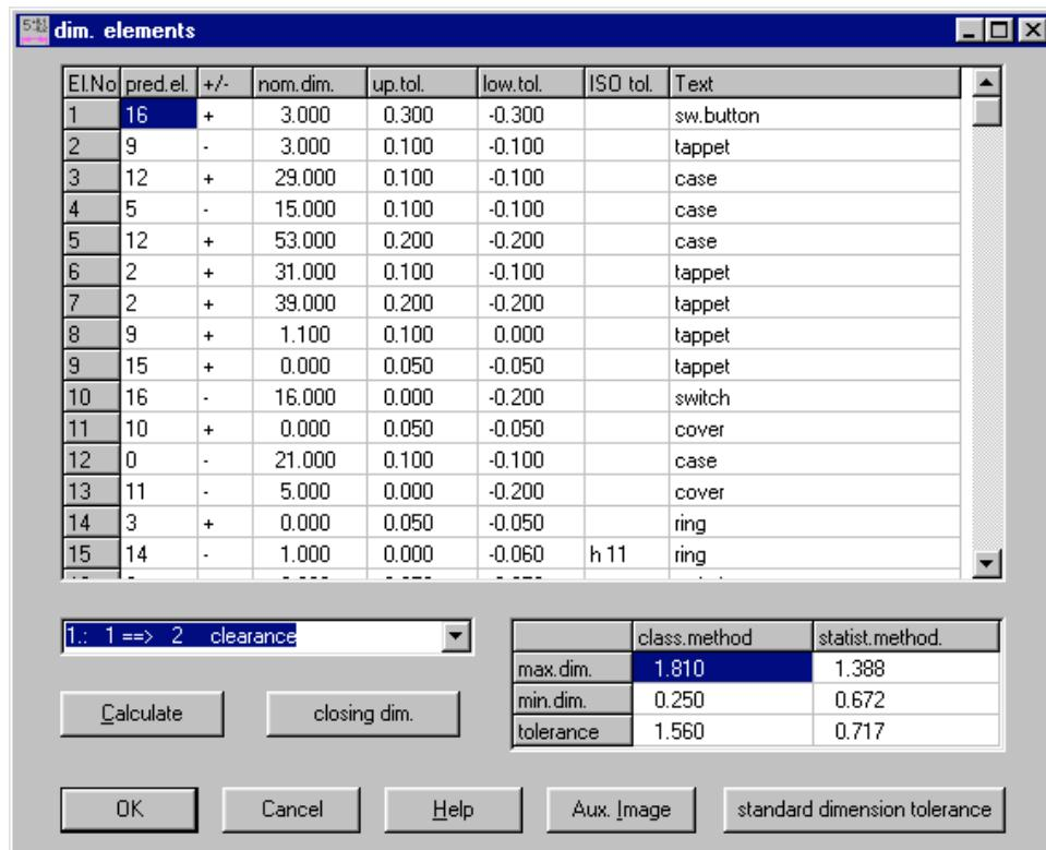
Next the critical distances are entered. For switch position "OFF" this is 1 => 2 and for position "ON" the distance 0 => 2.
