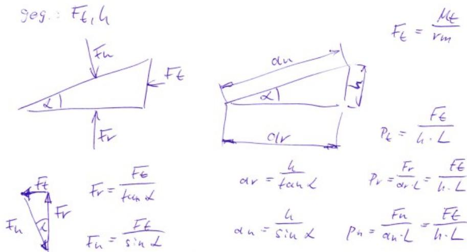
Let us consider the surface pressure on a wedge. One might expect the surface pressure to be highest where the force is greatest. In fact, the force and contact area are proportional, which is why the surface pressure on the wedge is the same everywhere:  $p = Ft / (h * L)$
