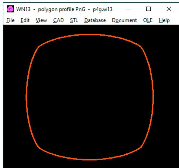
of teeth (P2G, P4G, P5G, P6G). WN13 thus replaces WN6, the calculation of dimensions and profile curve are identical. Surface pressure and minimum wall thickness are not calculated in accordance with DIN 32711, but in accordance with DIN 6892 (surface pressure parallel key connection) and DIN 7190 (minimum wall thickness of interference fit). Files from WN6 can be imported.
