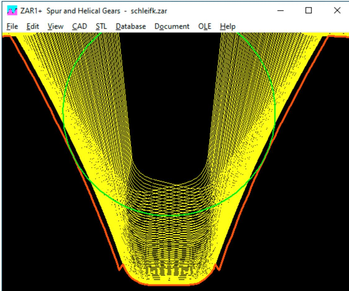
Once again a customer sent a tooth profile picture with an edge from the transition from the involute to the tooth root fillet with the question of whether this was a bug in the software. A check of his calculation file showed that a machining allowance  $q$  was entered, but a normal reference profile (no protuberance profile) was used. Then there are grinding notches, and these can also be seen in the tooth profile picture.
